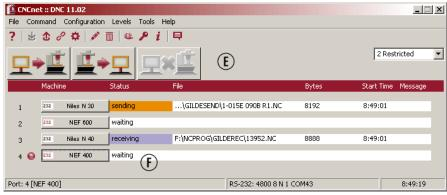
Every instance of the CNC network software (E) is able to control up to 100 machines simultaneously. The total number of installable instances is just limited by your computer. Different machine specific protocols like Heidenhain or Mazatrol are optionally available. The CNC network software is waiting (F) for remote commands from the control.
