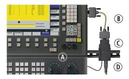
By using a short serial (RS232) cable (B) the control (A) gets connected to the added network adapter (C) and the network (D). The machine directly supplies the power for the adapter.
